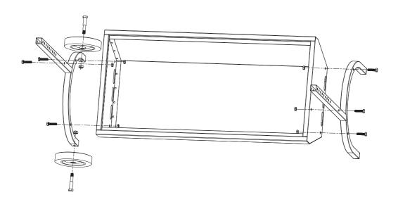
**Step 2**Slide the support assemblies onto the posts and secure with the fixing pin and split pin.
